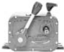
E Model 3 Torque Rating 12 in. lbs. Speed Range 400-0-400. Normal Input 1/4 - 1/3 H.P.
