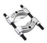
Features 'knife-like" edges which are easily placed behind the part to secure a gripping surface, even when clearances are extremely limited. When used with an OTC Grip-O-Matic® puller, puller jaws grip attachment's outer edge; when used with a Push-Puller, puller legs are threaded into the attachment's two tapped holes.
