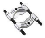
Features 'knife-like" edges which are easily placed behind the part to secure a gripping surface, even when clearances are extremely limited. When used with an OTC Grip-O-Matic® puller, puller jaws grip attachment's outer edge; when used with a Push-Puller, puller legs are threaded into the attachment's two tapped holes.
