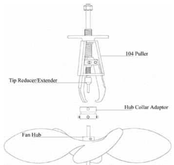
The collar adaptor secures the model 104 puller to hubs up to 3" in diameter. Set screws grip the hub and align the collar adaptor. The puller jaws are tightened securely into the hub collar groove eliminating slippage during fan and blower wheel removal.
