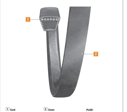
The cord is coated with a special compound that produces a secure, long-lasting bond with the surrounding rubber to assure longer life without separation problems. In addition, Blue Ribbon's dependable length stability means the belt requires significantly less re-tensioning and take-up.
